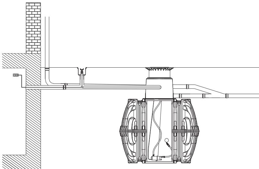
**Caution:** The distance between the water plug socket and the underground tank is limited by the pressure hose – length of the pressure hose is 10 m.
